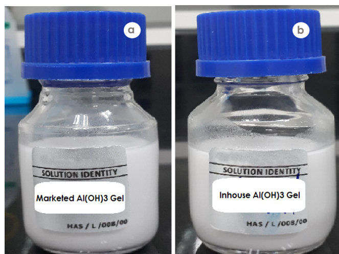
figure 25: Photographs of aluminum hydroxide suspensions. (a) Marketed formulation; (b) Formulation containing Natrosol™ 250 M Pharm HEC as a viscosity modifier.
