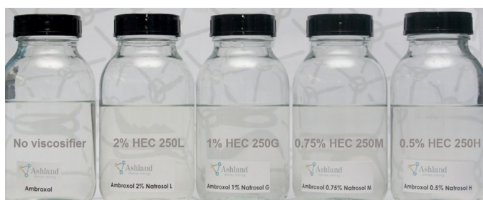
figure 16: Photographs of ambroxol formulations using varying amounts of different Natrosol™ 250 Pharm HEC grades.
