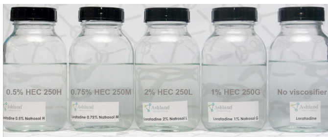
figure 18: Photographs of loratadine formulations using varying amounts of different Natrosol™ 250 Pharm HEC grades.
